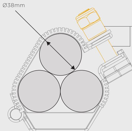
Nut spacer and partially threaded bolt prevent cable coming into contact with the thread
