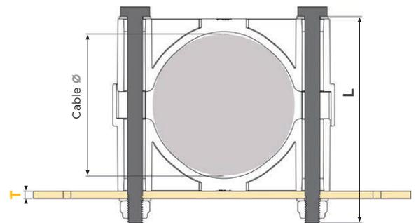
1 Bolt: Bolt Length (L) = Cable Ø + T + 48.0mm
