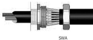
4. While continuing to push the cable forward to maintain contact between the armour and the cone, tighten the Nut (2) by hand to engage the armour. Hold the Entry Component (1) with a spanner and tighten the Nut (2) using a spanner until the armour is secured.
