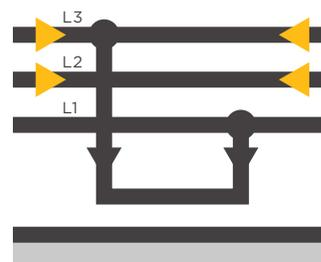
Fig 3. Phase-phase-to-earth short circuit
