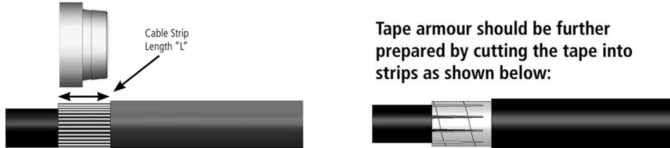
**Tape armour should be further prepared by cutting the tape into strips as shown below:**
