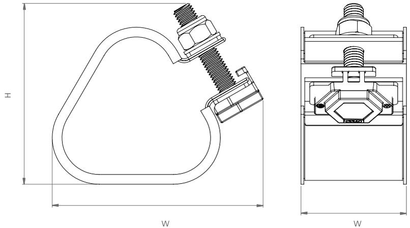
The CMP SDSSIR intermediate restraint range are metallic restraints which have been designed, constructed, and tested in accordance with the International Standard 'Cable Cleats for Electrical Installations' IEC 61914 to ensure the securing and retention of cables, without sustaining damage to the cable(s).
