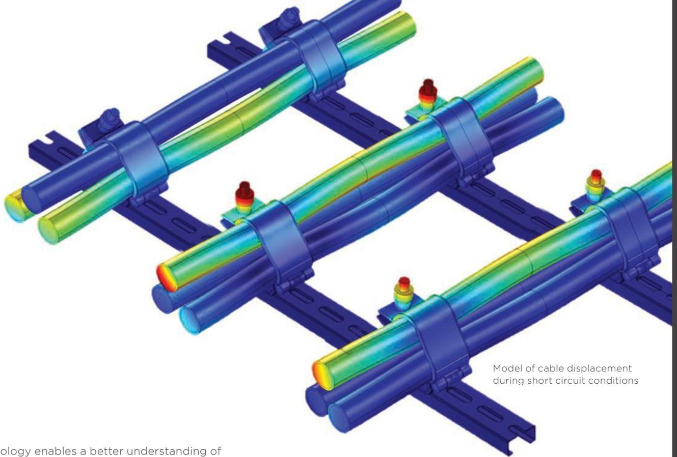
Model of cable displacement during short circuit conditions
