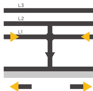
Fig 2. Phase-phase short circuit clear of earth
