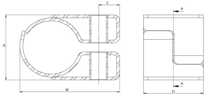
The CMP Products Helios Standard Duty, One Bolt, High Temperature Fire Rated Stainless Steel single cable cleat is a fabricated metallic cleat which has been designed, constructed, and tested in accordance with the International Standard 'Cable Cleats for Electrical Installations' (IEC 61914).
