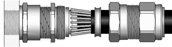
5. While continuing to push the cable forward to maintain contact between the armour and the cone, tighten the Main Item (2) until the inner seal makes contact with the cable inner sheath (heavier resistance is felt at this point). Tighten a further full turn. NOTE: The earthing device on E2\* type glands will automatically engage the lead sheath.
