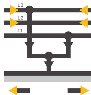
Fig 4. Three-phase short circuit
