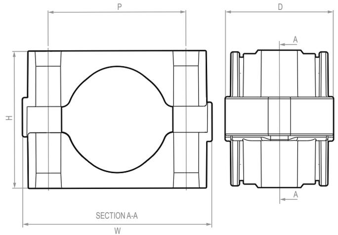
The CMP Products Themis Heavy Duty, Two Bolt, High Temperature Fire Rated Stainless Steel single cable cleat which has been designed, constructed, and tested in accordance with the International Standard 'Cable Cleats for Electrical Installations' (IEC 61914). It ensures the retention and securing of single cables, without damaging or deforming the cable.
