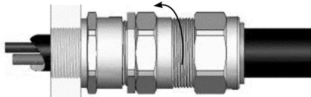
7. Only using finger pressure, tighten the outer seal nut assembly (6) until light resistance to tightening is met.
