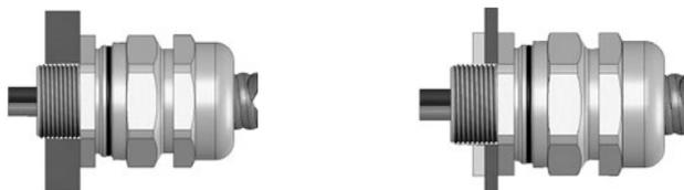
3. Loosen the body (4) and the outer seal nut (8) to relax the retaining spring (5) and seal jacket (7) respectively. (IT IS NOT NECESSARY TO SEPARATE THE COMPONENTS.)
