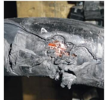
Major cable damage caused by thread contact
