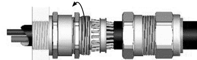
6. Hold the Main Item (2) with a spanner and tighten sub-assembly "B" onto sub-assembly "A" using a spanner until all available threads are used.
